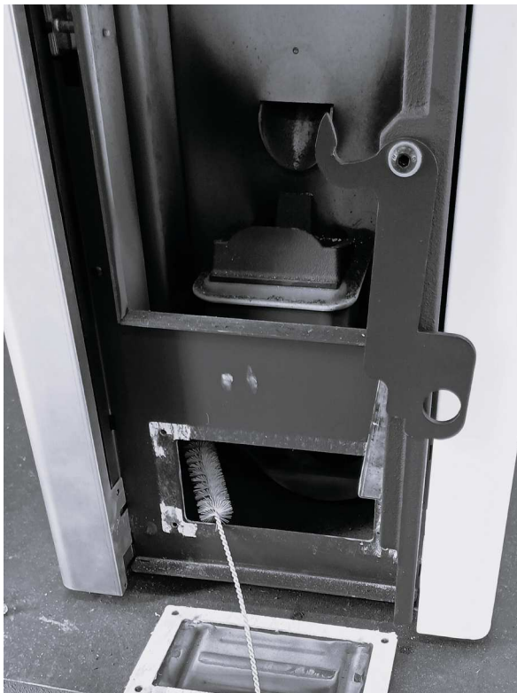
Fig. 28 - Clean with pipe cleaner
