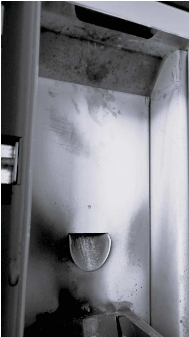
Fig. 22 - Remove the head of the firebox 1
